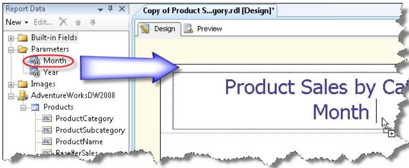
Figure 3.21 Create a placeholder by dragging a field from the Report Data pane.
