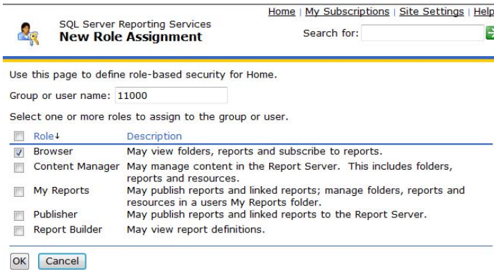
Figure 19.4 Use Report Manager to define for every user a role assignment that grants Browser rights to the Home folder.
