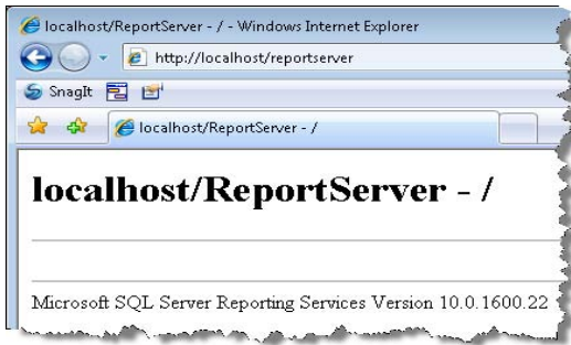
Figure 2.13 Request the Web Service URL to verify that the report server is operational.
