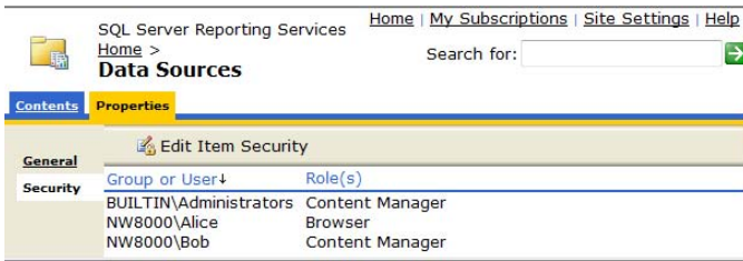
Figure 11.23 As a best practice, consider revoking end user access to the Data Sources folder.
