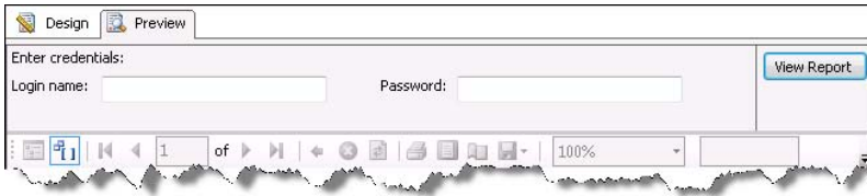
Figure 4.5 The Prompt for Credentials option generates Login Name and Password fields to collect credentials before the report is run.
