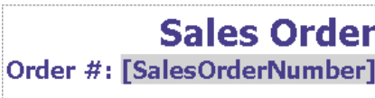
Figure 1.9 The textbox report item now supports multiple bands of text and each band can be formatted independently.
