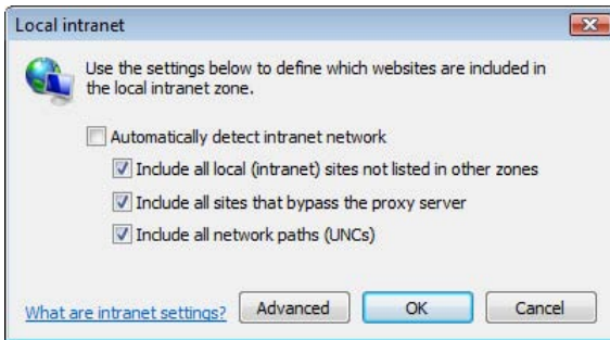
Figure 2.15 Configure the Local Intranet settings to suppress the credentials dialog with Windows Vista.
